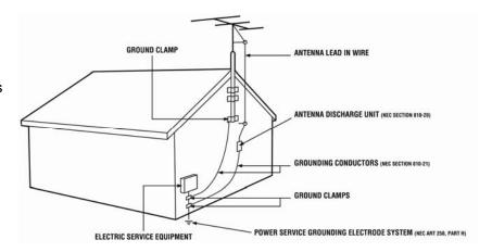
Remember, the screen of the coaxial cable is intended to be connected to earth in the building installation.
